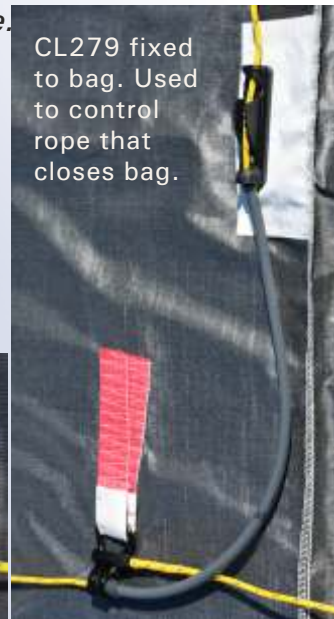
Usually 5 to 8 PT406 are fitted per bag, to guide the rope around the bottom of the bag.
