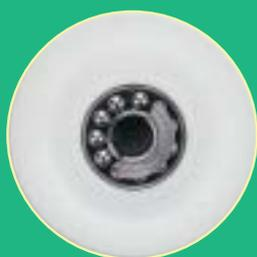
As you can see from the sectioned sheave the s/s balls work between two steel covers to share the load in a perfectly homogeneous way, avoiding this way, even under strong stresses, the making of impressions in the pulley and the ovalization of the balls.
