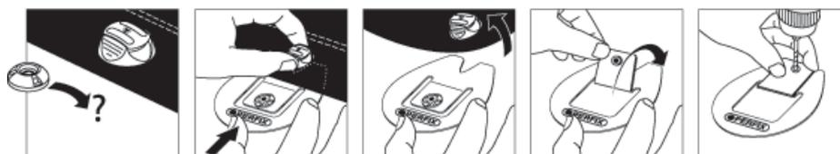
*By using the drill stencil you won't need to make any marks, the drill won't slide about and a lot of time will be saved (see illustration).*
