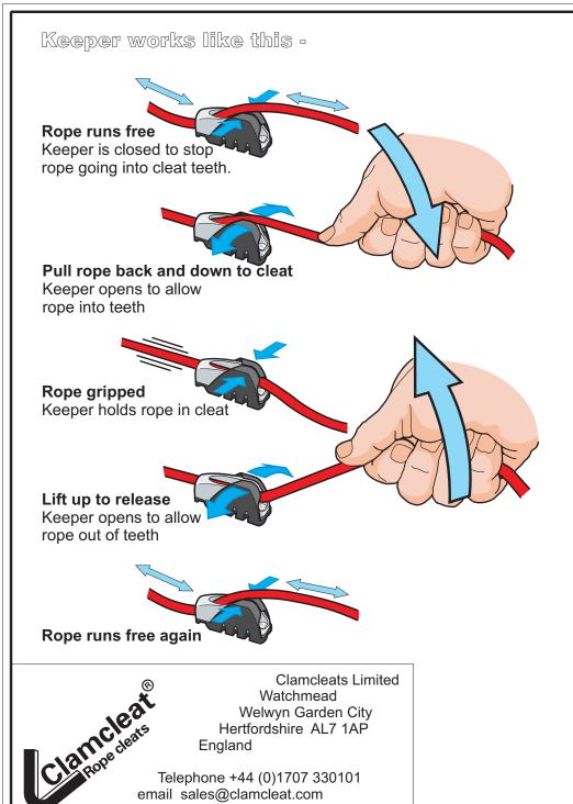
Rope runs free Stainless Steel rear fairlead guides rope down into teeth even when pulled at extreme angles. Rope gripped
